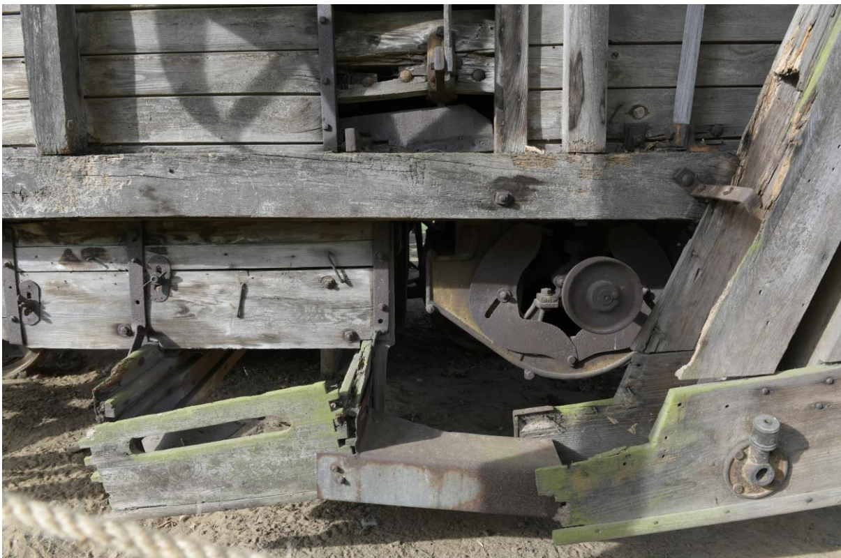
3. Lewa strona, elewator i wentylator
